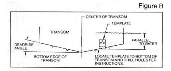
Once the location is determined mark and drill three 7/64" dia.. holes noted on the template. Attach the metal bracket using three #10 self threading screws supplied. Be sure to align holes in the center of the
