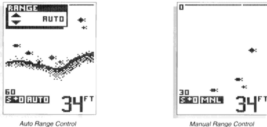
If you alter the depth range, Manual operation is automatically selected. This feature is valuable if you are only interested in targets near the surface. The LCR W will always display the digital depth of the water, regardless of whether the bottom is shown on the selected depth range.
