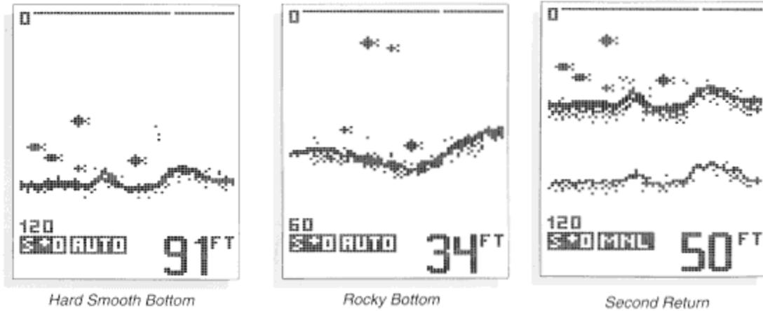
The transmitted sonar signal travels downward, and is reflected back toward the surface by the bottom or other objects for display on-screen. The signal does not stop there - it is reflected downward again by the surface of the water, and a weak "second return" is usually visible if the depth range is sufficient to see it. A second return is shown in the figure below. Some users use this second return as an indicator when setting the sensitivity bias.
