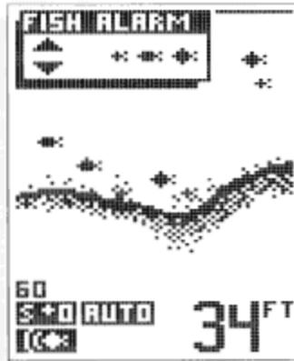
Remember that it is impossible for sonar to determine if a signal return is a fish or some other type of object or suspended debris. Any object not connected to the bottom is normally a fish and is portrayed as a fish symbol. The strength of the reflected sonar signal from a target is a good indicator of the size of the target, and the fish symbol displayed represents the strength of the signal reflected from it.
