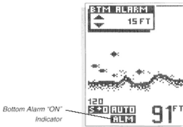
The LCR W contains an audible alarm to warn you of shallow water depths. This alarm is adjustable from 2' to 99' of depth. To enable the alarm, simply adjust the alarm depth using the UP and DOWN arrow buttons. When the depth of the water beneath your boat is equal to or less than the selected alarm depth, a continuous alarm will sound.
