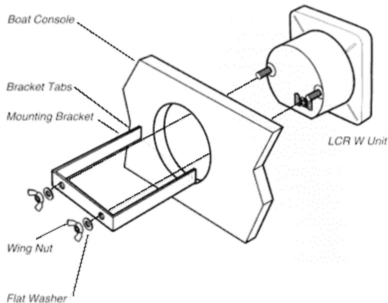
From the front of the console, place the unit into the 3.5" hole. Be sure that the unit's orientation reads properly before continuing.
