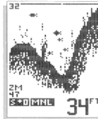
Pressing the UP or DOWN arrow button enables zoom and adjusts the zoom 'window' to the desired depth. The upper and lower limits are shown on-screen and the digital depth readout will continue to track the bottom even when Zoom is enabled.
