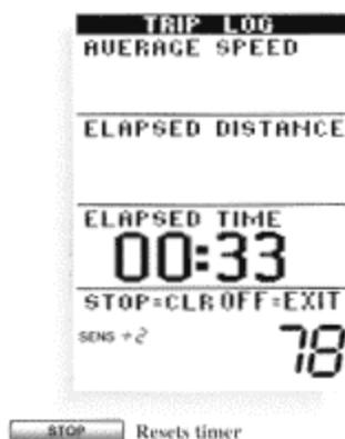
Although speed and temperature accessories are not available for the LCR 120, the Trip Log provides a useful timer. The timer begins when the unit is powered and can be reset and any time by pressing STOP. Pressing ON-OFF exits Trip Log and returns you to normal LCR 120 operations.
