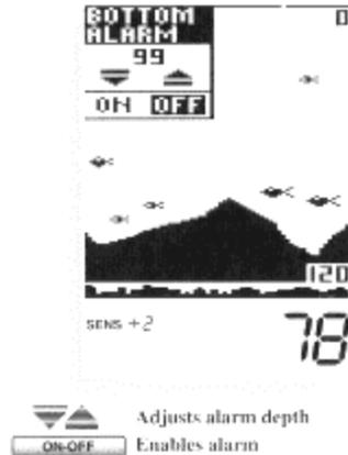
The Bottom Alarm lets you specify the minimum depth you want to maintain. To use it, select **BOTTOM ALARM**; then press the **ON-OFF** button to activate the alarm, and the Up or Down arrow button to adjust the depth at which the alarm depth when this function is on.
