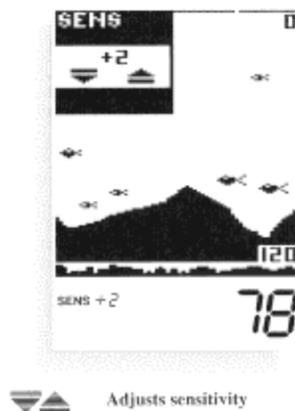
The LCR 120 automatically adjusts to the proper amount of sensitivity for conditions (i.e. depth). You can bias the setting + or -5 levels to suit your personal taste. Increasing the sensitivity targets and the thermoclines, which might not be displayed at the +0 setting. If you want to manually adjust Sensitivity, select SENS and press the Up or Down arrow button to adjust the display.
