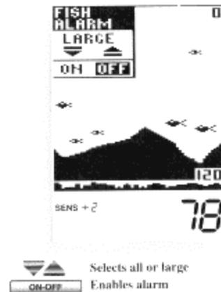
The Fish Alarm alerts you with a chirping sound whenever the LCR 120 detects fish (or another object not attached to the bottom). To activate it, select **FISH ALARM** and press the **ON-OFF** button.
