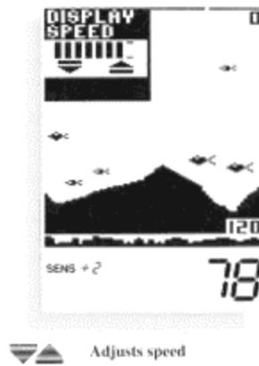
The LCR 120 display is “updated” (advances across the screen) as you move through the water. The speed at which the display is updated depends on the Display Speed setting. To adjust it, select DISPLAY SPEED, and press the Up arrow button for a faster setting or the Down arrow for a slower setting.
