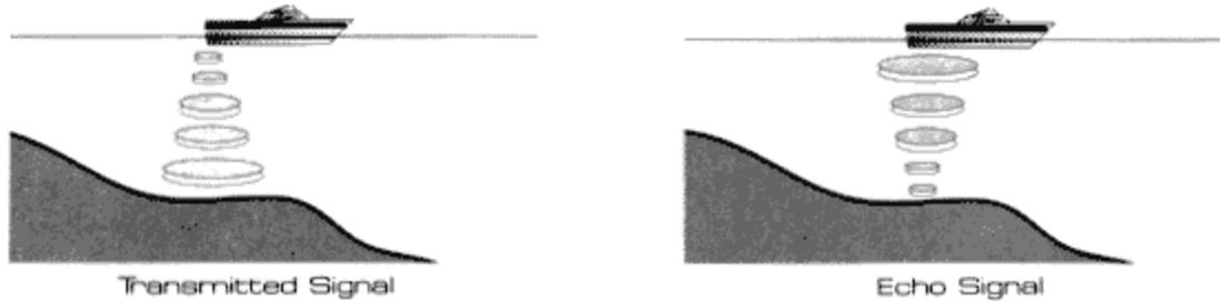
The transducer and LCR 100 use the basic principles of sonar to reveal objects beneath the water's surface. The LCR 100 continuously sends electronic signals to the transducer, which converts them to ultrasonic signals that it aims toward the bottom. Each signal travels downward until it strikes an object or the bottom, then immediately echoes back to the transducer. As the transducer receives these signals, it converts them back to electronic signals for display on the LCR 100 screen.
