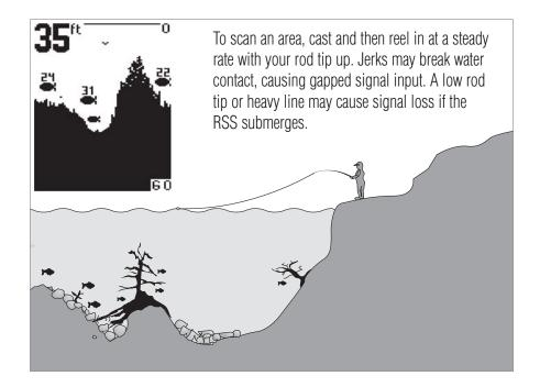
The returned "echoes" are transmitted with wireless technology to the display unit and plotted on the LCD. New information appears on the right. As this information moves to the left a very accurate picture of the underwater world is created, including the depth of underwater objects such as the bottom, fish, and structures.
