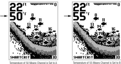
Temperature of 55 Means Channel is Set to B
