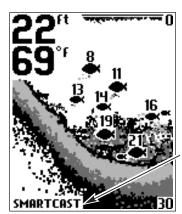
**SmartCast<sup>TM</sup>:** This user mode allows you to operate the PiranhaMax30 with an Advanced RSS.
