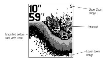
There is also a series of manual ranges which can be selected. The manual depth ranges are determined by the present depth conditions.
