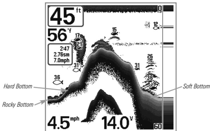
The sonar returns from the bottom, structure and fish can be represented as either **Inverse** (default), **WhiteLine®**, **Structure ID®**, or **Bottom Black**. See *Sonar X-Press™ Menu: Bottom View* for details on how to set the bottom view.
