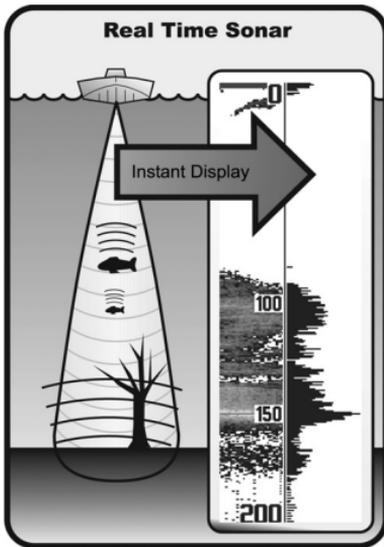
SONAR is an acronym for SOund and NAvigation Ranging. Sonar utilizes precision sound pulses or "pings" which are emitted into the water in a teardrop-shaped beam.
