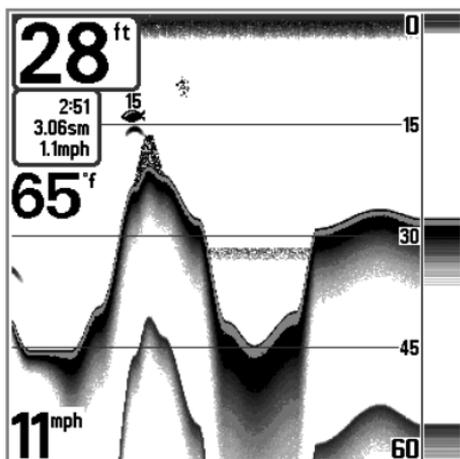
**Bottom Black** displays all pixels below the bottom contour as black, regardless of signal strength. This has the benefit of providing a high contrast between the bottom and other sonar returns on the display. Any targets such as fish, structure and thermoclines will be shown using the Structure ID® method.
