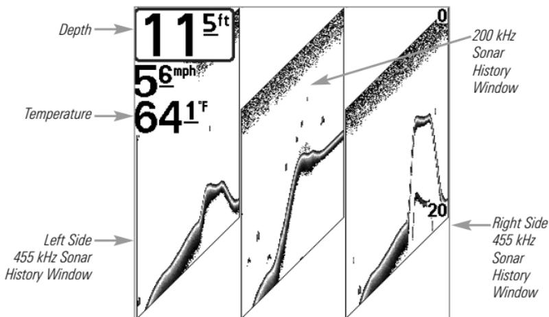
In all of these layouts, the sonar information from the side-looking beams reveals bottom contour, structure and fish similar to the down-looking beam, but the area covered is to the left and right of the area shown in the down-looking portion, so you actually see more of the bottom. The distance covered by the right and left beams is based on the depth setting for the down-looking beam, up to a maximum of 160 feet.
