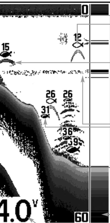
83 kHz, Wide Beam Hollow Fish Symbol
