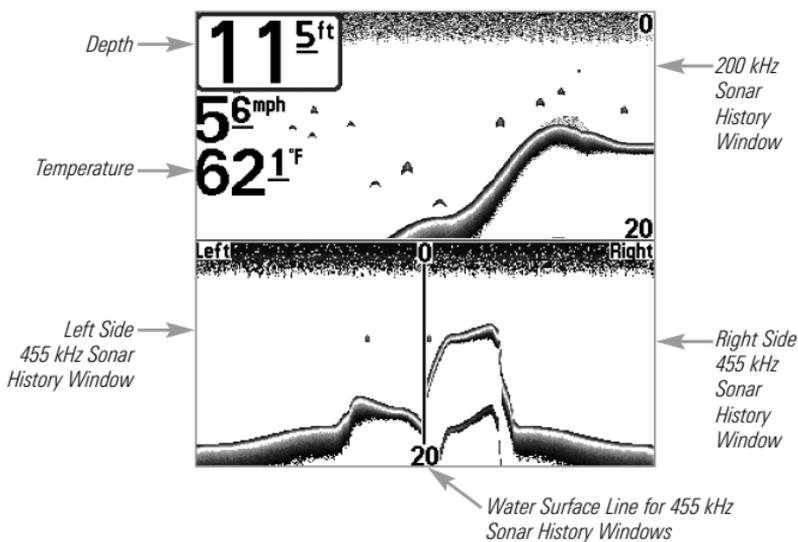
**Classic layout:** The top portion of the display presents a historical log of sonar returns from the 200 kHz down-looking sonar beam. The bottom portion of the display presents a historical log of sonar returns from the 455 kHz right- and left-looking sonar beams. New information appears at the top, and scrolls down the display.
