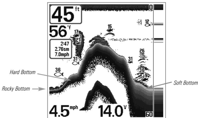
The sonar returns from the bottom, structure and fish can be represented as either **Inverse** (default), **WhiteLine®**, **Structure ID®**, or **Bottom Black**. See *Sonar X-Press™ Menu: Bottom View* for details on how to set the bottom view.
