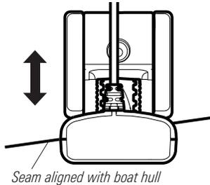
**NOTE:** The transducer has a natural downward slant of 4-5 degrees from leading edge (closest to the boat transom) to trailing edge (farthest away from the boat). Looking at the back of the transducer, the seam should be slightly below the bottom of the hull.
