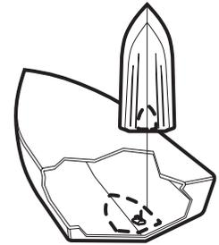
4. Fill the hull with enough water to submerge the transducer body. Use a sand-filled bag or other heavy object to hold the transducer in position. The transducer cannot transmit through air, and the water purges any air from between the transducer and the hull, and fills any voids in the coarse fiberglass surface.
