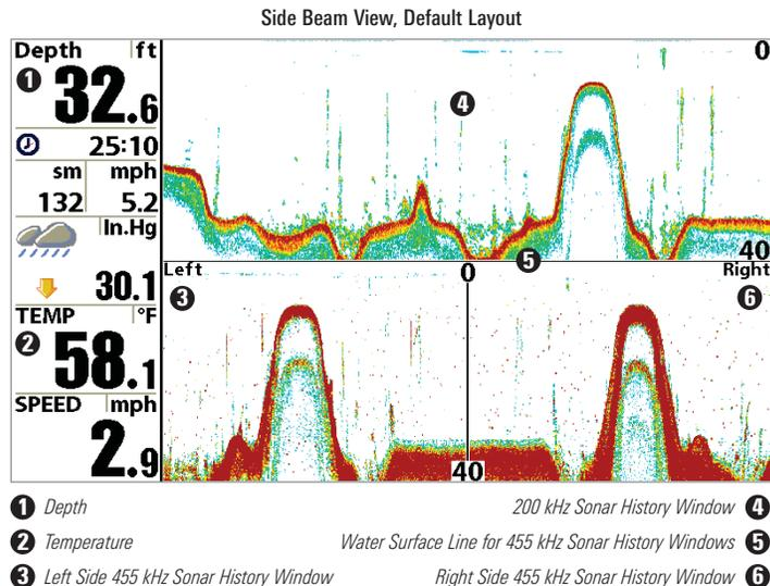
**Classic layout:** The top portion of the display presents a historical log of sonar returns from the 200 kHz down-looking sonar beam. New information in the down beam panel scrolls from right to left. The bottom portion of the display presents a historical log of sonar returns from the 455 kHz right- and left-looking sonar beams. New information appears at the top, and scrolls down the display.
