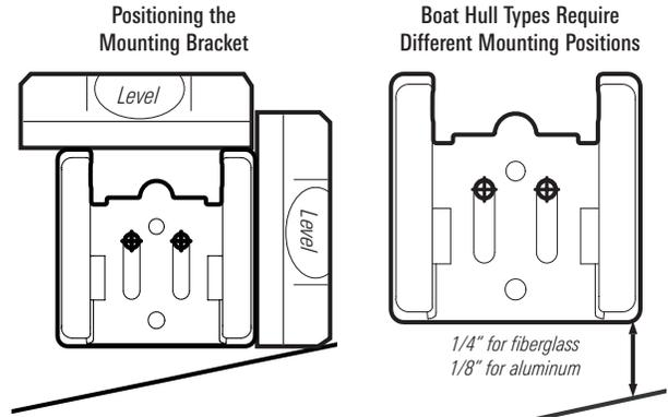
**NOTE:** If you have a flat-bottomed aluminum boat, some additional adjustment may be needed to accommodate the rivets on the bottom of the boat (i.e. the gap may need to be a little smaller than 1/8"). This will help you to avoid excessive turbulence at high speeds.
