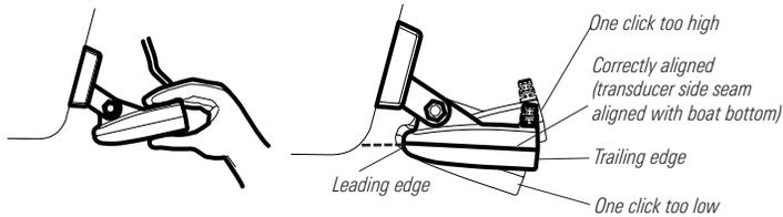
7. Adjust the transducer assembly vertically, until the seam on the leading edge of the transducer (the edge closest to the transom of the boat) is level and just slightly below the hull.
