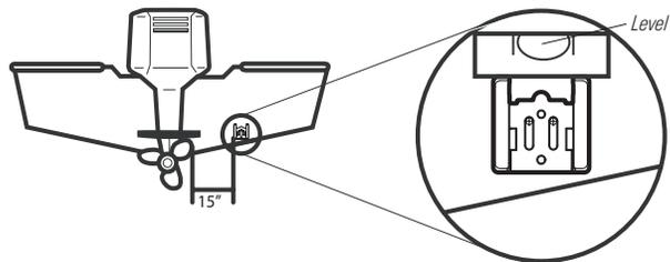
Find a turbulence-free location at least 15" from the propeller(s) and not in line with trailer bunks or rollers.
