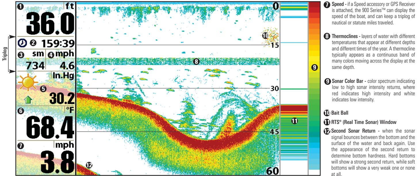
**7 Speed** - if a Speed accessory or GPS Receiver is attached, the 900 Series™ can display the speed of the boat, and can keep a triplog of nautical or statute miles traveled.
