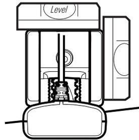
8. Continue to adjust until the bracket is also level from port to starboard (horizontally level as you look at the transducer from behind the boat).
