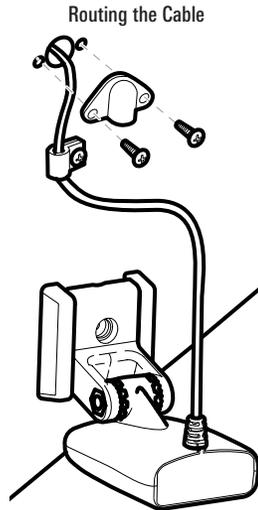
4. Route and secure the cable by attaching the cable clamp to the transom; drill one 9/64" diameter x 5/8" deep hole, then fill hole with marine-grade silicone sealant, then attach the cable clamp using a #8 x 5/8" screw.
