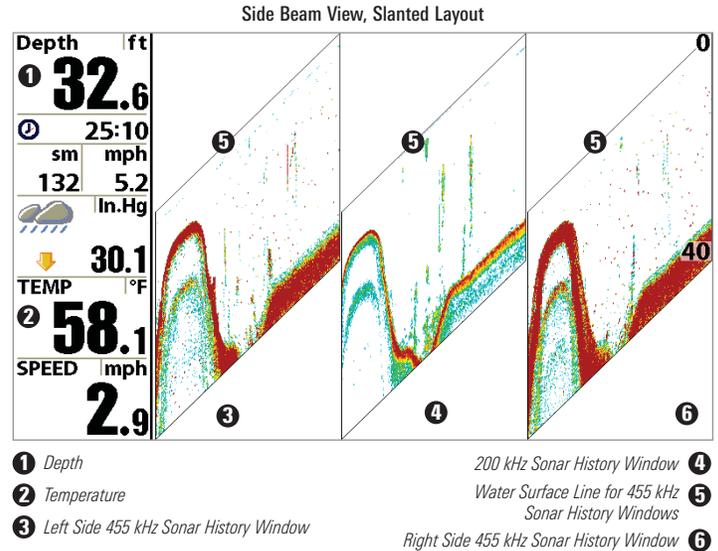
In all of these layouts, the sonar information from the side-looking beams reveals bottom contour, structure and fish similar to the down-looking beam, but the area covered is to the left and right of the area shown in the down-looking portion, so you actually see more of the bottom. The distance covered by the right and left beams is based on the depth setting for the down-looking beam, up to a maximum of 160 feet.
