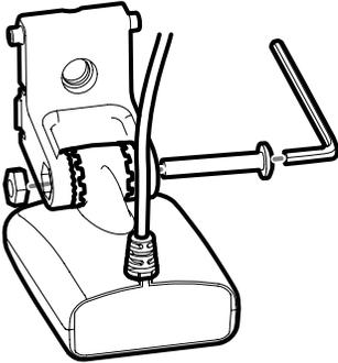
Inserting the Pivot Arm Assembly Into the Mounting Bracket
