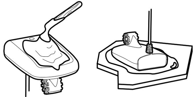
5. Coat the face of the transducer and the inside of the hull with epoxy.
