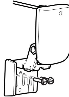
**NOTE:** Make sure that the mounting screws are snug, but do not fully tighten the mounting screws at this time to allow the transducer assembly to slide for adjustment purposes.
