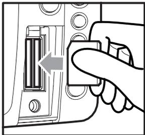
Inserting an MMC/SD
