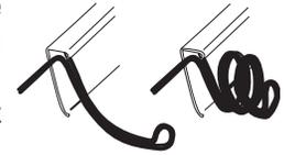
**NOTE:** If there is excess cable that needs to be gathered at one location (as shown in the illustration), dress the cable routed from both directions so that a single loop is left extending from the storage location. Doubling the cable up from this point, form the cable into a coil. Storing excess cable using this method can reduce electronic interference.
