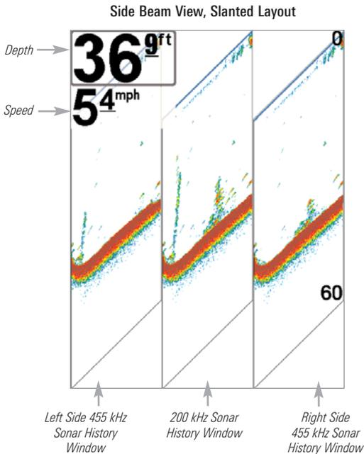
In all of these layouts, the sonar information from the side-looking beams reveals bottom contour, structure and fish similar to the down-looking beam, but the area covered is to the left and right of the area shown in the down-looking portion, so you actually see more of the bottom. The distance covered by the right and left beams is based on the depth setting for the down-looking beam, up to a maximum of 160 feet.
