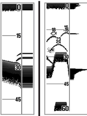
The **Wide RTS® Window** indicates the sonar intensity through the use of a bar graph. The length of the plotted return provides an indication of whether the return is weak or strong. The depth of the sonar return is indicated by the vertical placement of the return on the display depth scale. The Wide RTS® Window does not make use of grayscale.
