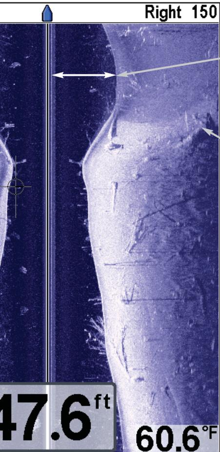
The **water column** shows the relative depth of the water under the boat at a given time. Variations in the width of the water column show variations in the distance to the bottom as the boat passes over.
