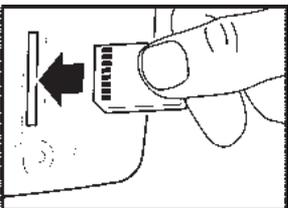
Inserting an MMC/SD
