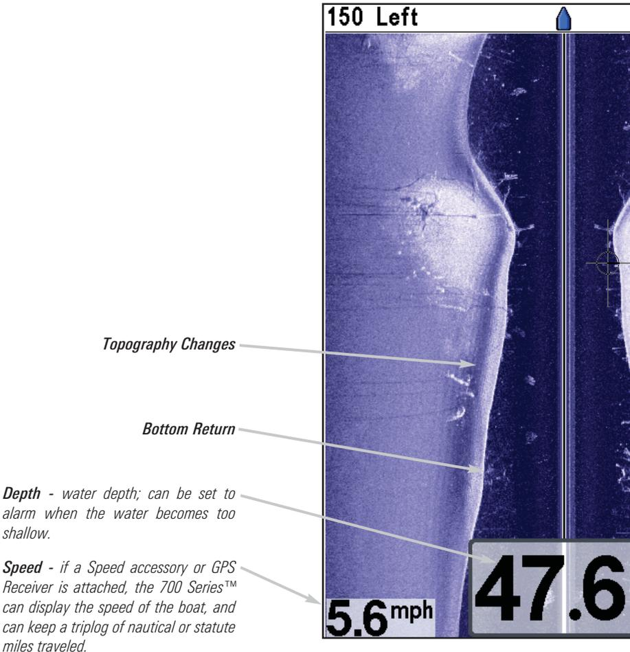
low for accurate interpretation of bottom contour and structure. For Side Imaging, the bottom rock and gravel provide a clearer sonar return than mud and sand because of their relative density. Hard slopes that face away from the transducer. You can find a number of easily recognizable features of bottom contour and structure, including the following items:
