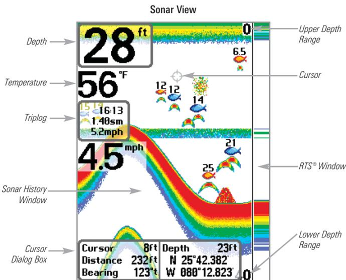
**NOTE:** If the Depth number is flashing, it means that the unit is having trouble locating the bottom. This usually happens if the water is too deep, the transducer is out of the water, the boat is moving too fast, or for any other reason that the unit can't accurately receive continuous data.
