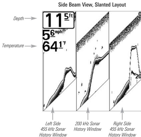
In all of these layouts, the sonar information from the side-looking beams reveals bottom contour, structure and fish similar to the down-looking beam, but the area covered is to the left and right of the area shown in the down-looking portion, so you actually see more of the bottom. The distance covered by the right and left beams is based on the depth setting for the down-looking beam, up to a maximum of 160 feet.
