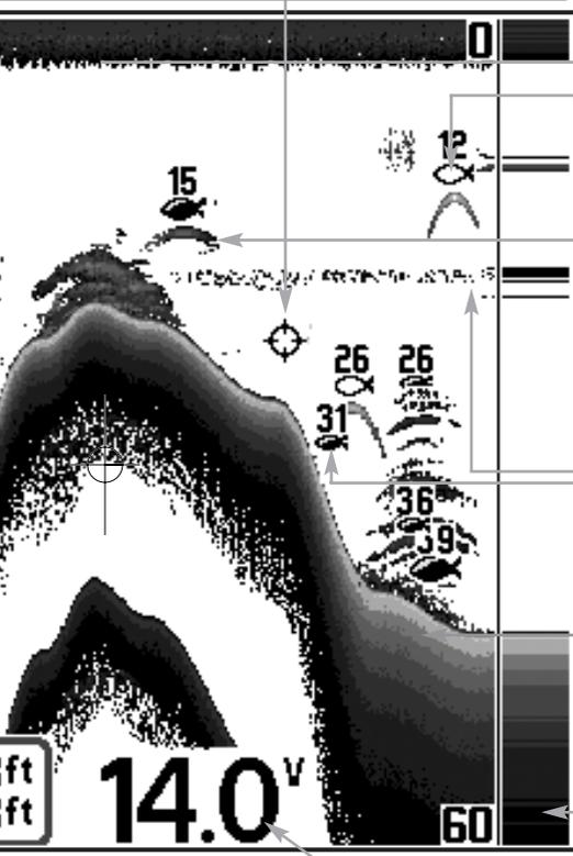
**83 kHz, Wide Beam Hollow Fish Symbol**
