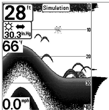
**NOTE:** To get the full benefit of the Simulator, it is important to select Simulator manually from the Start-Up Options menu as opposed to letting the Fishing System enter Simulator automatically (as it will if a transducer is not connected and you do nothing during power up). Manually selecting Simulator from the Start-Up Options menu allows you to pre-configure your Fishing System for on the water operation. Any menu changes you make will be saved for later use.
