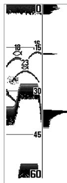
The **Wide RTS® Window** indicates the sonar intensity through the use of a bar graph. The length of the plotted return provides an indication of whether the return is weak or strong. The depth of the sonar return is indicated by the vertical placement of the return on the display depth scale. The Wide RTS® Window does not make use of grayscale.
