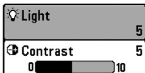
Your Fishing System will start up with the backlight on and will automatically turn it off to conserve power. To turn the backlight on for night fishing, or to adjust the display contrast, press the POWER/LIGHT key to access the Light and
