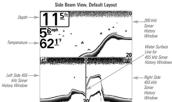
**Classic layout:** The top portion of the display presents a historical log of sonar returns from the 200 kHz down-looking sonar beam. New information in the down beam panel scrolls from right to left. The bottom portion of the display presents a historical log of sonar returns from the 455 kHz right- and left-looking sonar beams. New information appears at the top, and scrolls down the display.
