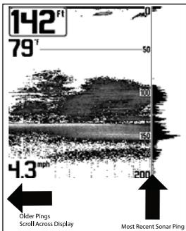
When all the echoes are viewed side by side, an easy to interpret "graph" of the bottom, fish and structure appears.
