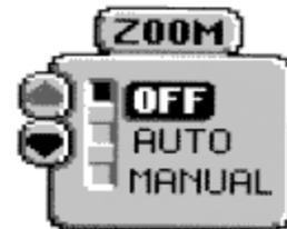
The Zoom ranges available are dependent on the current depth range. In the 15' (5m) depth range, TruZoom displays a range equal to one half the current depth range. In the 30' (10m), 60' (20m), 120' (40m), 180' (60m), 240' (80m), 360' (110m), 480' (150m) and 600' (185m) depth ranges, TruZoom displays a range equal to one fourth the current depth range. The box at the right side of the screen outlines the area to be zoomed.
