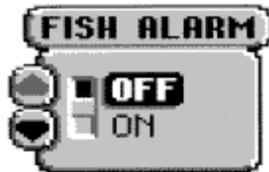
**Fish Alarm.** The Fish Alarm alerts you to the presence of fish, or other targets not connected to the bottom. The Fish Alarm has three different settings that correspond to the three different size fish symbols shown onscreen.
