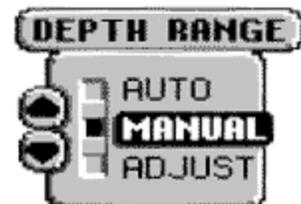
The Depth Range can be adjusted manually. Press MENU repeatedly until the Depth Range menu is visible. Two options are available: Auto and Manual.
