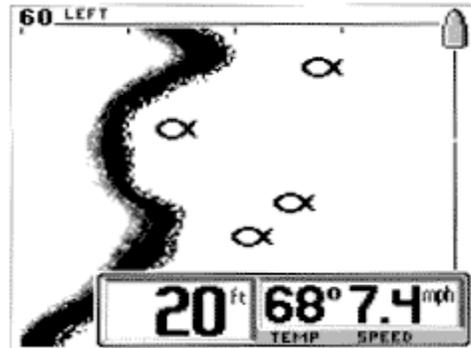
When operating in Wide Side mode, the range must be adjusted manually, since the bottom is often not visible on-screen. Ranges of 15 (5m), 30' (10m) , 60' (20m) and 120' (40m) are available. Also, Zoom is not possible in Wide Side mode, and the Zoom menu is not available.
