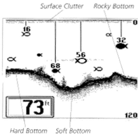
Wave action also affects the bottom depiction. The information drawn is a distance measurement, so if the boat is moving up and down over flat bottom, the bottom depiction often appears in regular variations that match wave timing.
