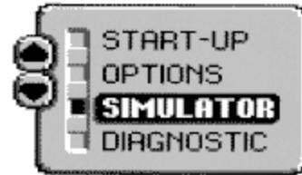
The simulator can also be started by selecting the Simulator option on the start-up screen after you power-up the unit. When this screen is shown, simply press the DOWN ARROW until "Simulator" is highlighted. When the screen times out, the unit will be in simulator mode.
