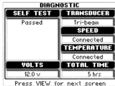
If you are using multiple transducers, switch between transducers to confirm the connections for each.
