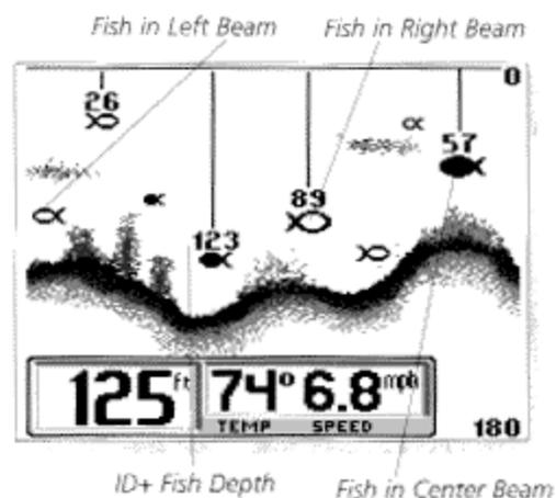
**ID+** adds an additional piece of information to help the user locate fish. On selected fish symbols, the digital depth of the designated fish is drawn to help locate the fish vertically. This is especially helpful in setting bait depths or for downrigger operation.
