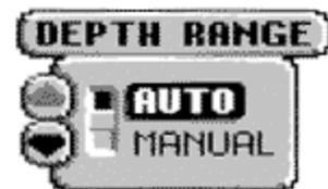
The 400TX automatically adjusts the depth range depending on the depth of the water. The unit tries to maintain the bottom depiction about 2/3 down the total range (for example, in 20' (6m) of water, the 0-30' (0-10m) range would be selected). This provides the best display resolution and therefore the best target separation possible.
