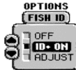
ID+ On enables the 400TX to interpret the raw sonar data and, using a variety of techniques, depict appropriate target returns as one of three different size fish symbols. Further identification shows which beam the fish is detected in. The 400TX also displays the depth beneath the surface with the corresponding fish symbol.
