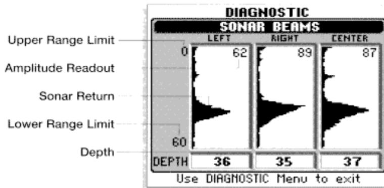
By referring to this screen prior to permanently mounting a through-the-hull transducer, the location can be adjusted until no visible loss is observed.
