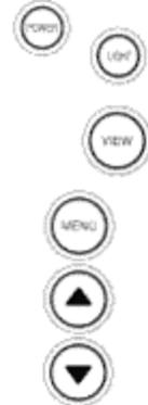
**Power.** The Power button powers the 400TX up for normal operation. When the unit is on, POWER turns the unit off. POWER can also be used to go directly into Simulator mode. To enter simulator, with the unit powered off, press and hold POWER for several seconds until a continuous chirp is heard.
