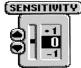
The user has the option of adjusting the Sensitivity higher or lower based on personal preference. You can select one of 11 sensitivity settings from -5 to +5. A setting of 0 (factory setting) has no effect on the automatic sensitivity control. Increasing the sensitivity (+1 through +5) enables the unit to display the information from progressively smaller sonar returns. By decreasing the sensitivity (-1 through -5), the unit effectively filters small sonar returns.
