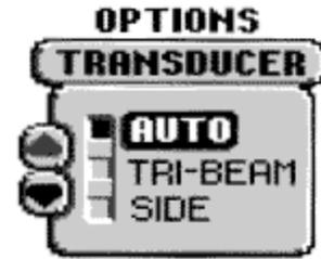
If a faulty transducer is connected, the 400TX may not change the screen presentation to match the transducer. In this instance, you may need to manually select "Tri-beam" for the tri-beam transducer or "Side" for the WideSide transducer.
