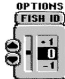
Selecting Adjust and making incremental changes enhances the fishfinder's ability to identify sonar returns as fish symbols.
