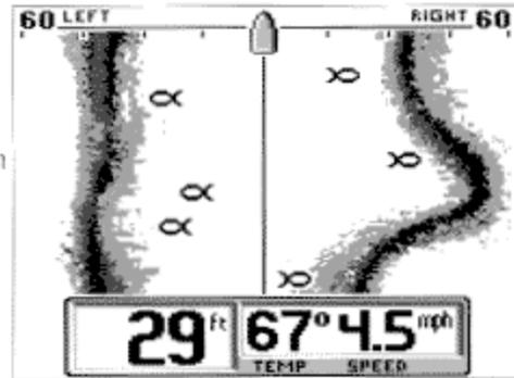
Viewing both left and right sides simultaneously gives you an excellent tool when searching for bait fish in open water, or when following a creek bed. However, you will have a greater display resolution if you view only one side.
