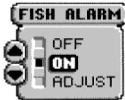
The default setting is "OFF." With the "Large fish only" setting, the 400TX alarms on only those targets that are represented by the large fish symbols. The 400TX can be set to alarm on only large and medium fish, or set to alarm on all fish.
