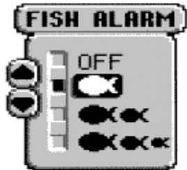
Once the Fish Alarm is enabled, the 400TX emits an audible beep when the selected size fish symbol appears on-screen. The sound is slightly different for each of the three fish symbol sizes, so with practice, it is possible to distinguish the size of the detected fish without looking at the unit.
