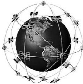
GPS uses a constellation of 24 satellites that continually send radio signals to the earth. Your present position is determined by receiving signals from up to 16 satellites and measuring the distance from the satellites.
