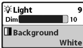
To adjust the backlight or to adjust the display background color, press the POWER/LIGHT key to access the Light and Background menu. Use the 4-WAY Cursor key to select Light or Background and then use the LEFT or RIGHT Cursor key to change the settings. Press EXIT to exit the Light and Background menu.
