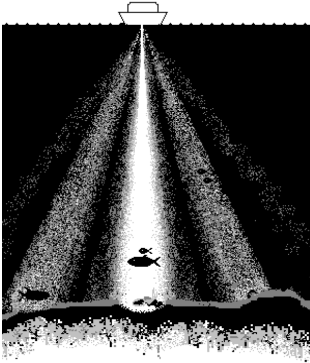
Figure 4. Bottom SONAR beam (cross-section)
