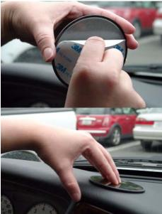
4. Attach the windshield mount to the adhesive disk by frimly pressing the suction cup against the disk. Lock the suction cup by pressing the locking lever.
