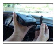
Slide the windshield mount onto the back of the cradle.
