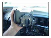
Press the windshield mount to the glass and slide the locking lever toward the glass.
