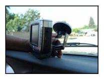
Plug the power cable and FM antenna into the Magellan RoadMate 6000T as shown. Use the suction cups to position the FM antenna along the windshield.
