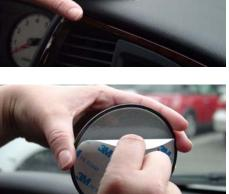
3. Apply the disk to the cleaned surface.
