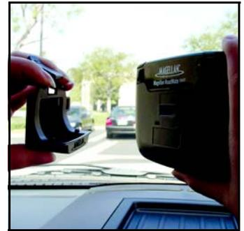
Slide the windshield mount onto the back of the car holder.
