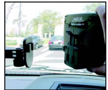
Press the windshield mount to the glass and slide the locking lever toward the glass.
