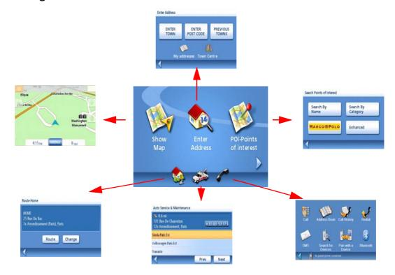
**Show Map:** Displays the map with your current position (if computing a position from the GPS signals) indicated by the blue triangle. See the Map Screen chapter for details.
